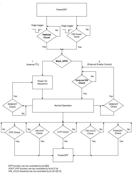
Figure 1. Power ON/OFF Flow Chart
