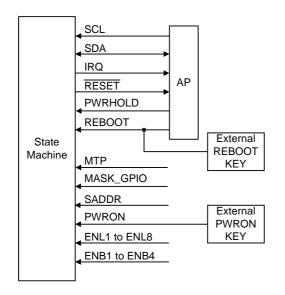
As MTP connect to AGND Inhibit to write MTP. As MTP connect to VIN Permit to write MTP.
