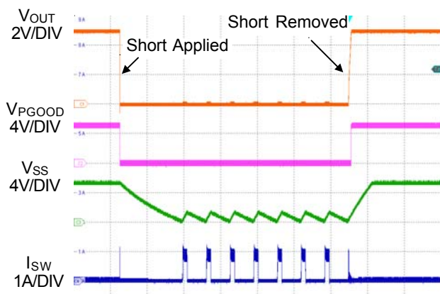
Figure 3. Short-Circuit Protection and Recovery
