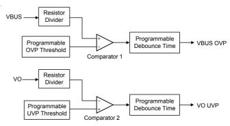
Figure 1. Functional diagram of VBUS OVP and VO UVP
