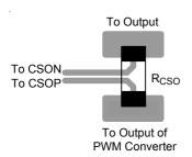
Figure 6. Kelvin connections for the R<sub>CSO</sub>
