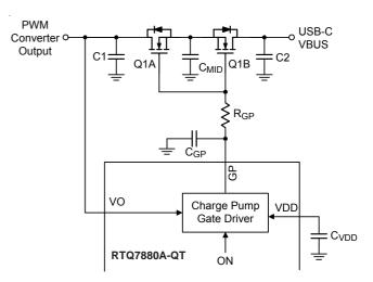
Figure 4. Functional diagram of the power-path control
