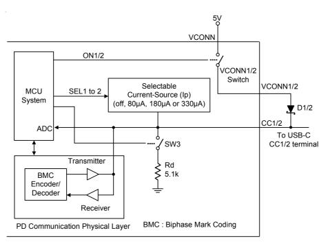
Figure 2. Functional diagram of VCONN and CC1/2 functions
