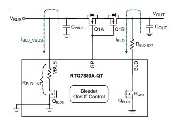
Figure 3. Functional diagram of the output bleeders
