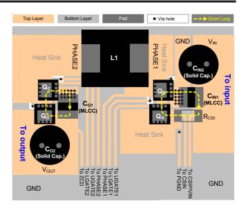
Figure 7. Recommended PCB layout of the power stage
