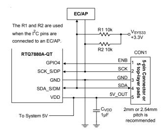
Figure 8. Connections for manual firmware updates
